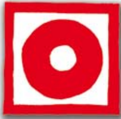
Manual alarm call point
