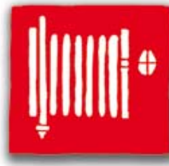
Equipped Fire Hydrant or BIE
