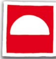
This sign shows where the fire fighting equipment is
