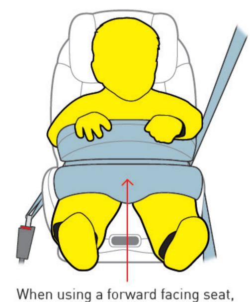
the shield slightly reduces the forcé exerted on the child when decelerating very quickly
