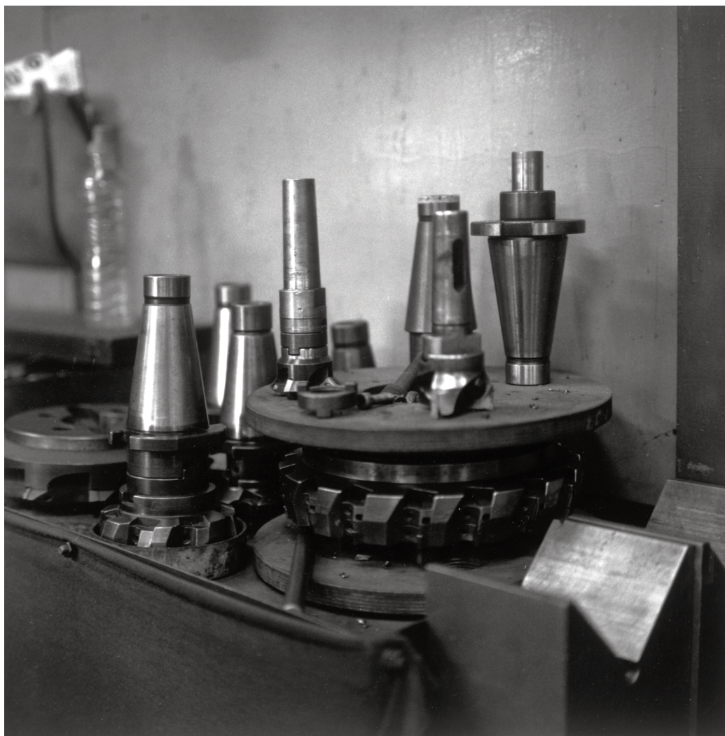
Portaherramientas de fresadora Zayer. From the series “Anonymous Labour. Iracheta SL, Can Ricart, Poblenuu, June-July 2005”. 2005
